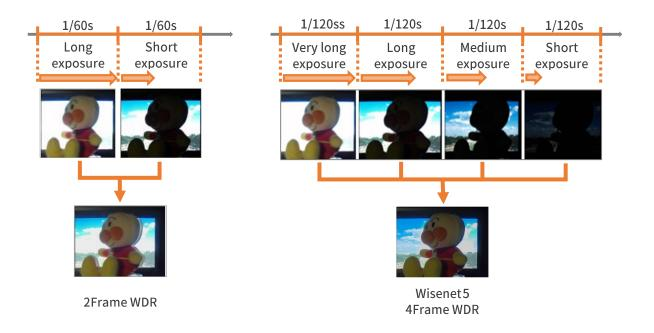
Figure 5. Comparison of the existing 2 fps WDR and 4 fps WDR applied to X series
