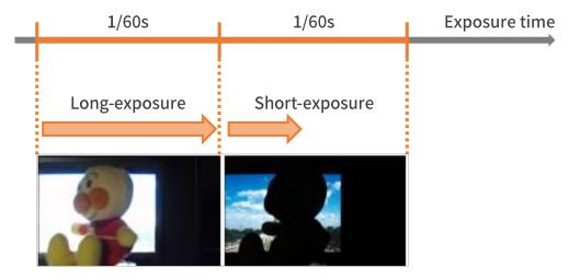
Figure 2. Process of obtaining long-exposure and short-exposure images
