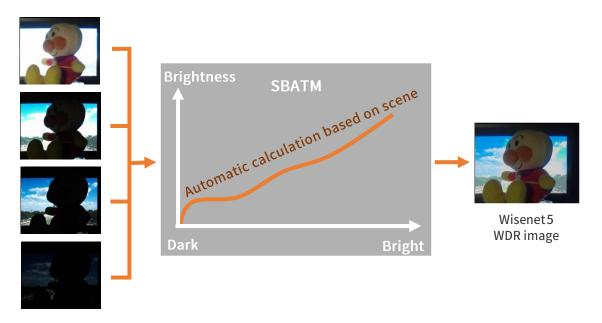
Figure 6. Process of generating an image in ultra wide dynamic range environment
