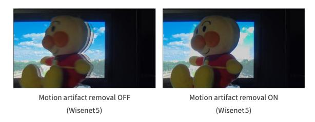
Figure 7. Effect of Motion Artifact Removal in an X series (Wisenet 5) product
