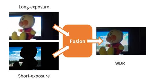
Figure 3. Process of composing long-exposure and short-exposure images
